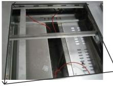
3. Wipe clean the Silicone Strips with isopropyl alcohol. Then place the Strips around the frame. Do not overlap the strips.
